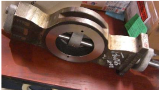
4 CL600x300 Wafer CF8M Natural Gas Shut Off Application
