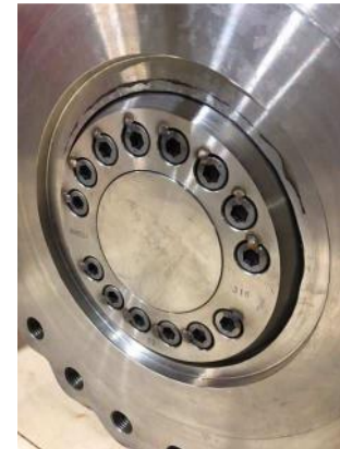
12 CL600 Lug CF8M x Stellite 21 High Vibration Flow Control Application
