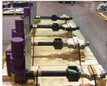
8 CL150 Lug CF8M Fire Isolation Valves Extension Heat Shield & KMASS Actuator
