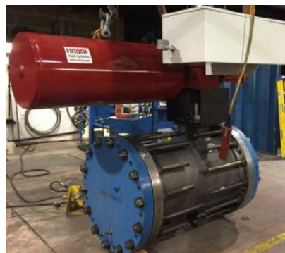
30 CL300 DF Gate WCB Electro Hydraulic Test Actuator Pressure and Cycle
