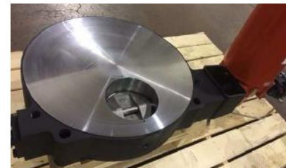
24x8 CL150 Wafer WCB Flow Control Application
