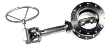
12 CL150 DF Gate CF3M Cryogenic NASA LOX Shutoff
