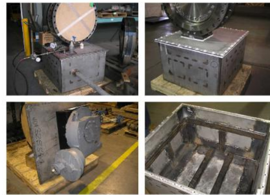
30 CL150 DF Short CF8M Submersible Actuator Enclosure
