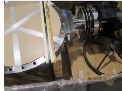
30 CL150 Lug CF8H High Temp Heat Ext Sulfuric Acid Service
