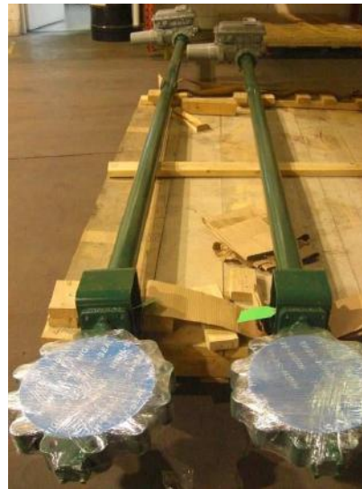
12 CL150 Lug WCB Highseal MOV 1 Actuator Extension
