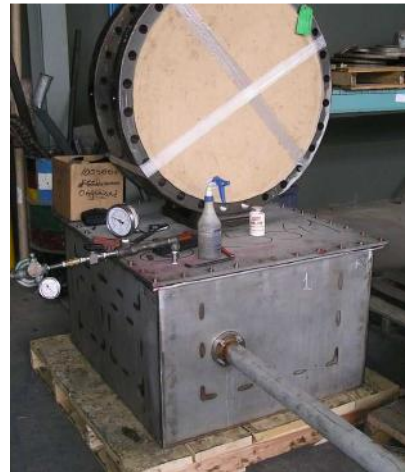
30 CL150 DF Short CF8M Submersible Test Actuator Enclosure Pressure
