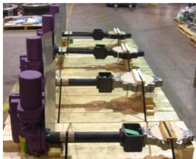
8 CL150 Lug CF8M Fire Isolation Extension Heat Shield & KMASS Actuator
