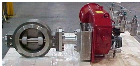
16 CL600 Wafer High Temperature Heat Extension
