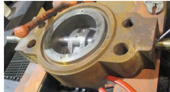
6 CL1500 x 300 RTJ Wafer WCB Control Application at Maintenance
