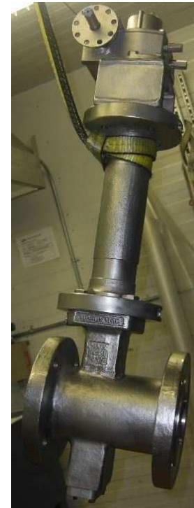
3 CL150 DF Gate CF3M Cryogenic NASA LOX Shutoff
