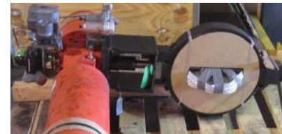
16x14 CL150 Wafer WCB Steam Jacket Body & Traced Shaft Fail Open
