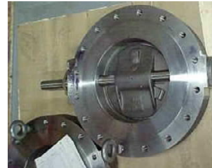
18 CL150 Lug Titanium Grade 2 Sulfuric Acid Service Mine Application
