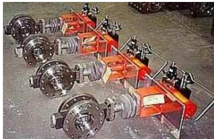
8 CL300 DF Short CF8MH High Temp Heat Ext Heat Shield Actuated
