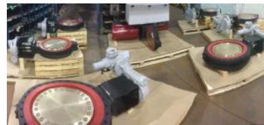
24 Wafer and 30 Lug CL150 WCB w/ Impreglon Coating x NiAlBz Trim Recycle Water
