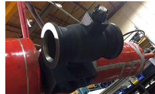
10 CL1500 WCB Clamp End Valve Refinery Compressor Application
