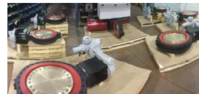
24 Wafer and 30 Lug CL150 WCB with Impreglon Coating x NiAlBz Trim Recycle Water
