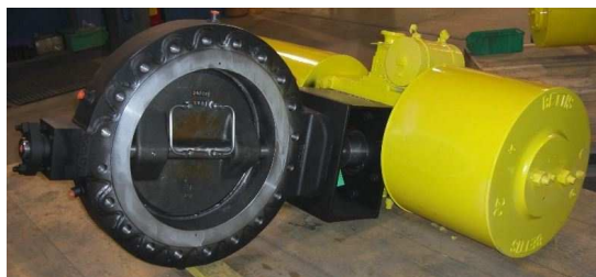
20 CL150 Lug WCB Jacket Body & Disc w/ Shaft Tracing
