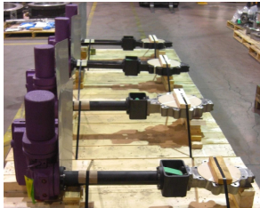
Actuator Extended with Heat Shield & KMASS 8 CL150 Lug Fire Iso.
