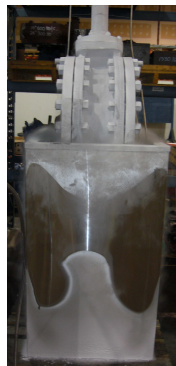
Gear Extension 36 Feet on 12 CL150 Lug WCB
