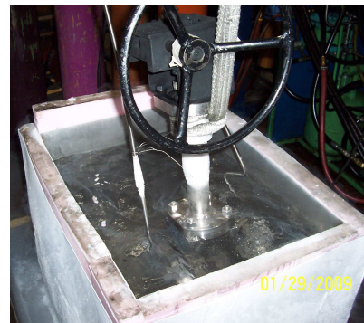
Cryogenic Testing 12 CL150 DF CF8M NASA
