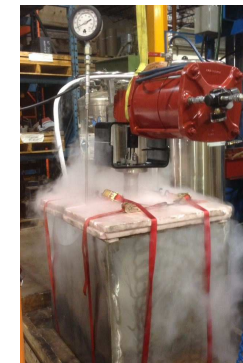
Cryogenic Testing 8 CL300 Lug CF8M Blue Origin
