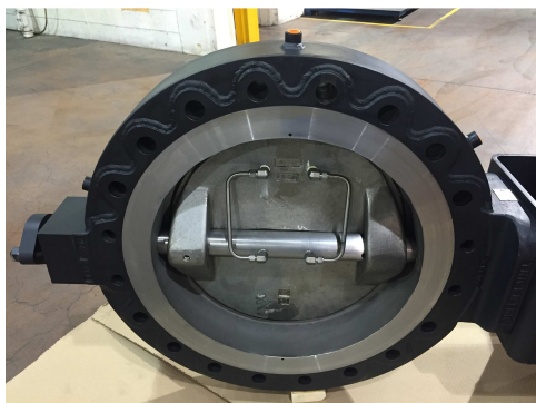
24 CL150 Lug WCBxCF8M Jacketed & Bleed Purge Disc
