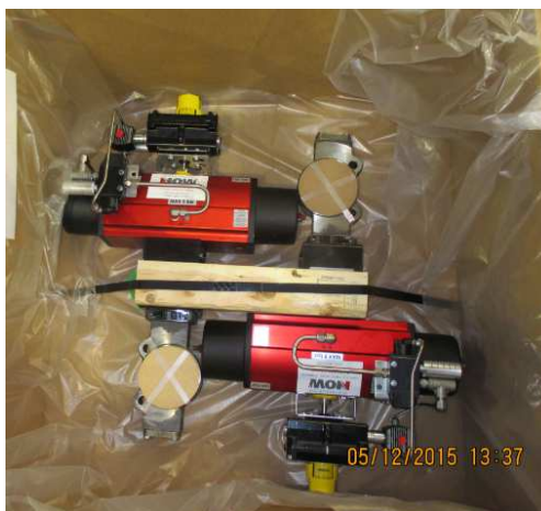
3 CL150 Wafer CF8M Actuated Control Application
